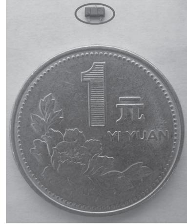
Fig. 1. p-i-n diode with model number mot\_bal99lt1.
